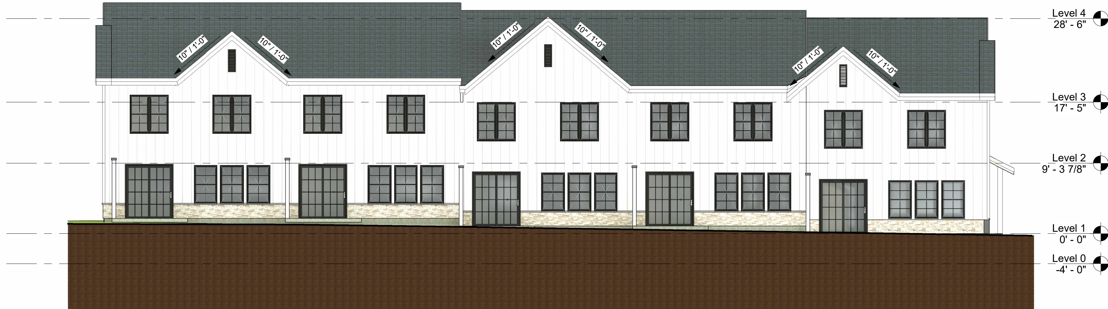
2 NORTH ELEVATION A2.0 1/8" = 1'-0"
